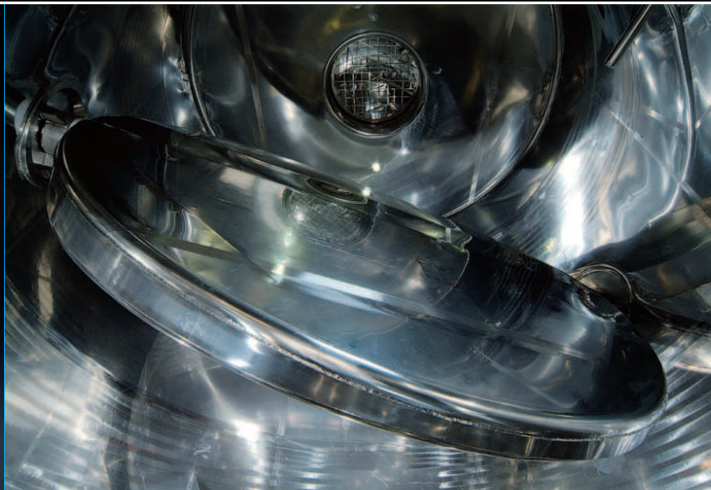
Full disk rotating blade patented by Albrigi, temperature-controlled on both sides
