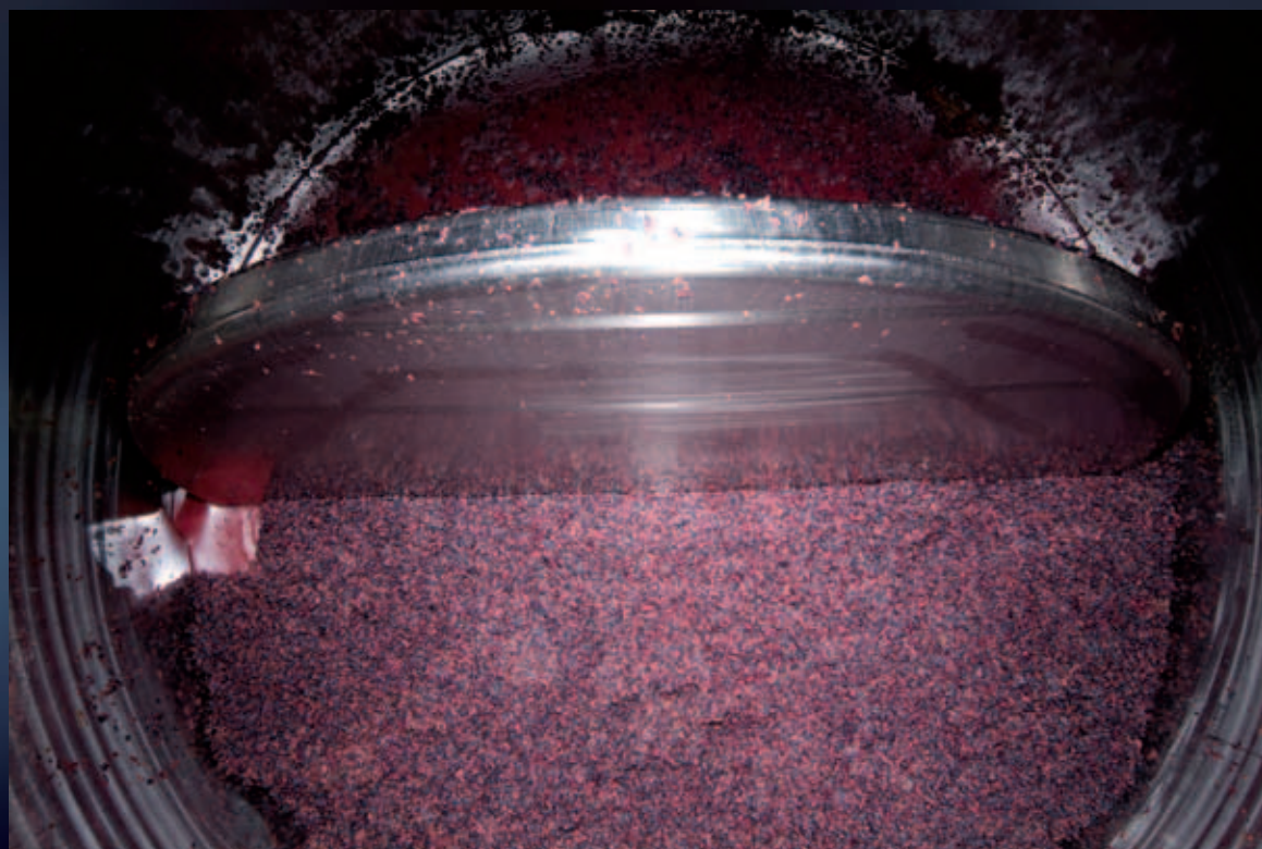
Vertically positioned rotating blade patented by Albrigi, with dry-raisin marc during a pause in the work cycle
