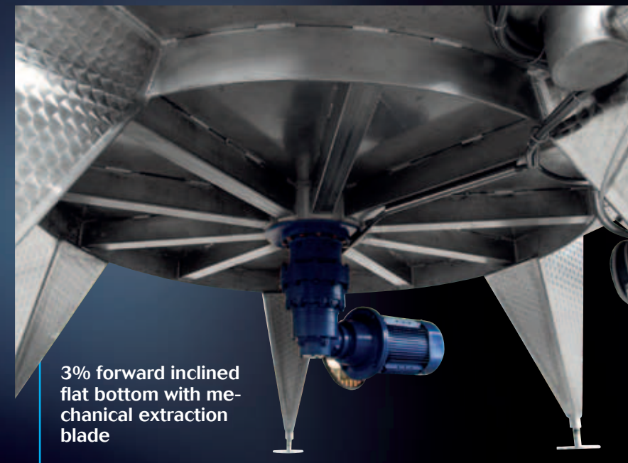
3% forward inclined flat bottom, temperature-controlled by Termostar
