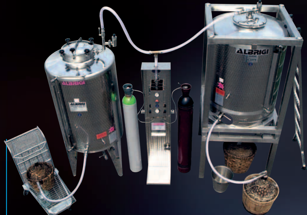
1000 liter insulated Enopalet tank with nitrogen gas system and 1000 liter "S" series Minitank
