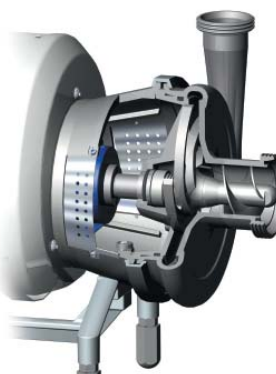
Special version equipped with an inducer in the suction port. This device is fitted immediately upstream of the impeller to reduce the NPSH required by the pump.
