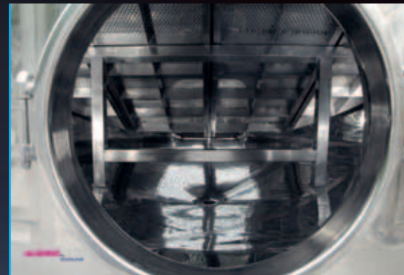
Inside view of the lower part of the dripping grate through the lower hatchway
