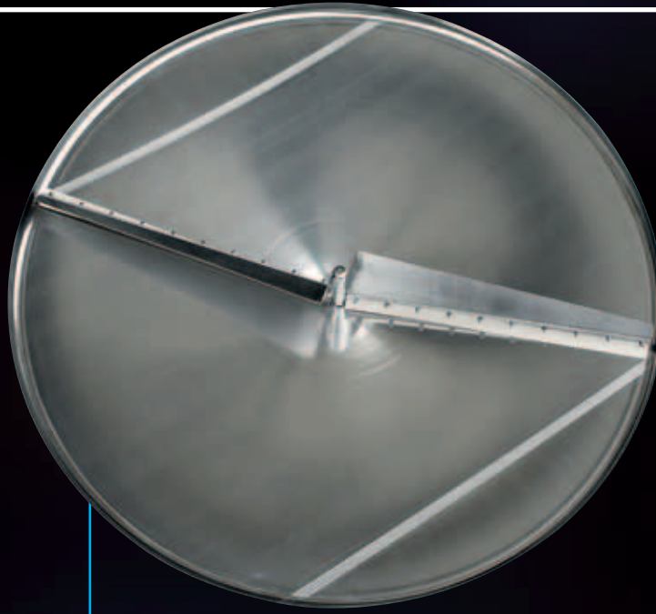
View of the rotating Bâtonnage blade on the bottom
