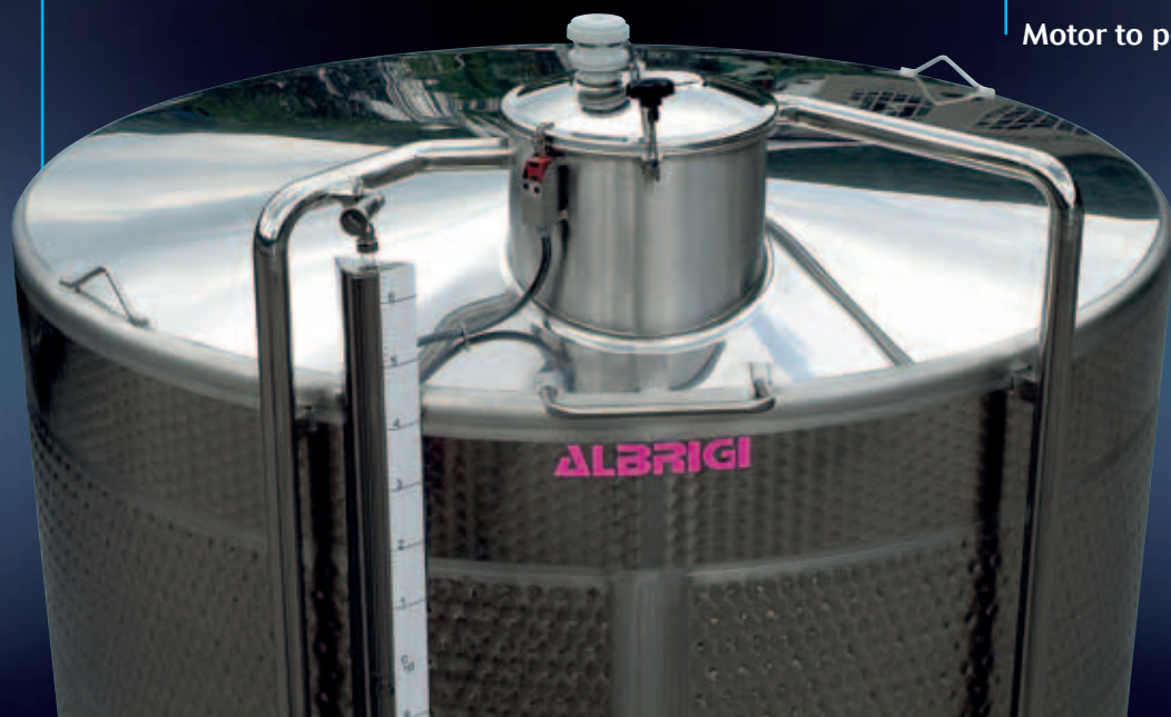
View of the front manhole cover with pumping over and the Cleanfix washing plant
